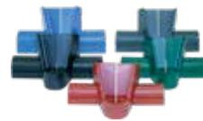
Truss Rod Hose Slings securely fasten a 3/4" flexible hose to the truss rod to maintain drop/sprinkler position. Supporting the flexible hose of the drop prevents kinking and abrasive wear. Color-coded models are available for various truss rod sizes: 5/8" (rust), 1/6" (green), 3/4" (black), 13/16" (grey), and 7/8" (blue).
